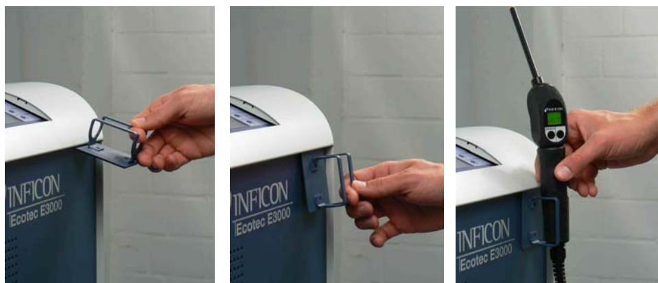
Fig. 9: Sniffer line holder mounting
