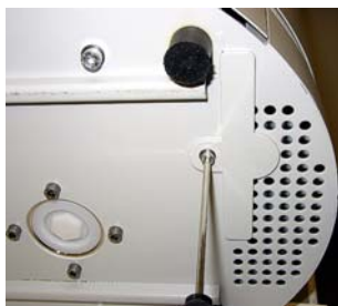
Fig. 48: Loosening the air filter cover
