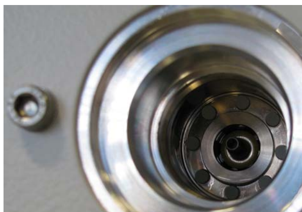
Fig. 52: Porex rods of the operating fluid reservoir
