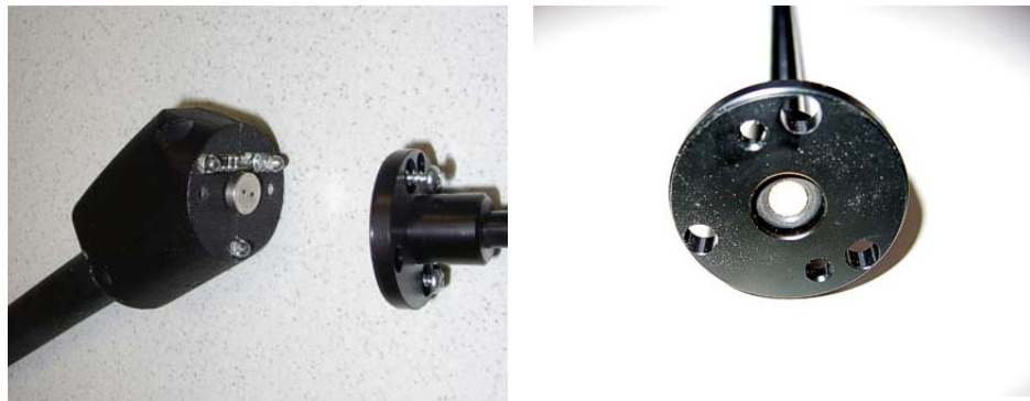
Fig. 57: Sinter filter in the sniffer handle
